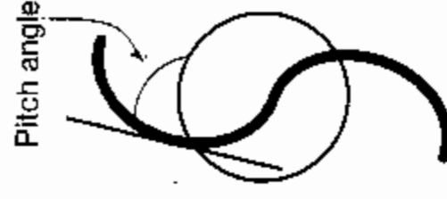
FIGURE 2.8 Pitch angle is measured at a given radius from a circle to the tangent of the arm.
