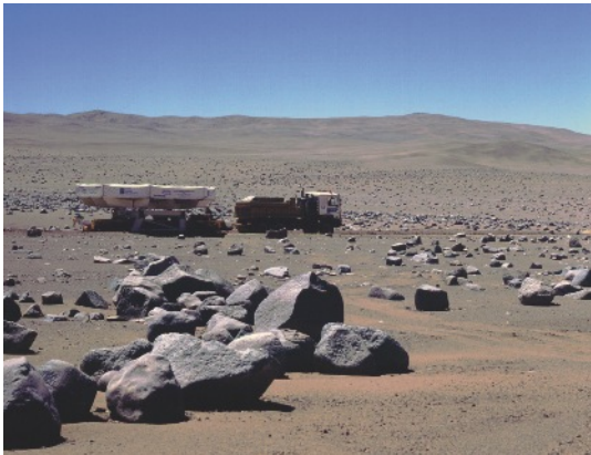
Fig. 1.30. Left: Transport of one of the VLT mirrors from Antofagasta to Paranal. The route passes through an extremely dry desert, and large parts of the road are not paved. The VLT thus clearly demonstrates that astronomers search for ever more remote locations to get the best possible observing conditions. Right: The active optics system at the VLT. Each mirror is supported at 150 points; at these points, the mirror is adjusted to correct for deformations. The primary mirror is always shaped such that the light is focused in an optimal way,
