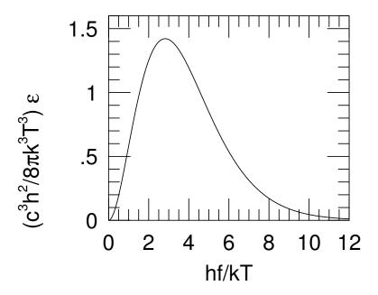
Figure 2.7: The energy distribution of a blackbody spectrum.
