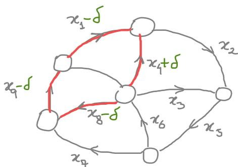
$$c_1(x_1 - \delta) + c_4(x_4 - \delta) + c_8(x_8 - \delta) + c_9(x_9 - \delta) \\ c_1 x_1 + c_4 x_4 + c_8 x_8 + c_9 x_9 + \delta \underbrace{(-c_1 + c_4 - c_8 - c_9)}_{> 0}$$
